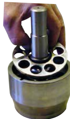
14. Remove the retaining plate.
