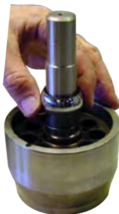
15.Remove the retaining ball.
