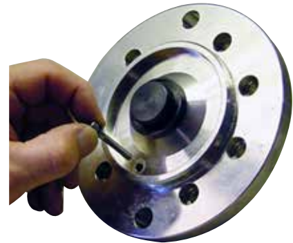
20. Mount the washer and the screw in the front flange to fix the swash plate.
