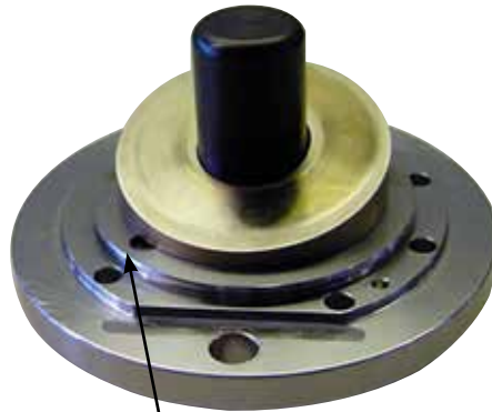
19. Mount the O-ring on the front flange.
