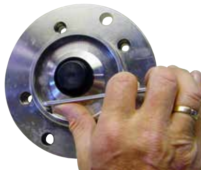
21. Tighten the screw to a torque of 8 Nm and remove the tool.
