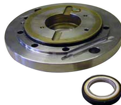
18. The ceramic ring removed from the front flange.
